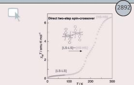
Direct two-step spin-crossover through [HS–HS][LS–LS] at the plateau in dinuclear diiron(II) complex [{Fe(NCBH\_3)(4phpy)} $_2$ (µ-bpypz) $_2$ ]
