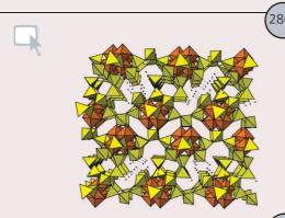
A germanium zeotype with a three-dimensional net of interconnected 14-, 12- and 12-ring channels.  $Ge_{13}O_{26}(OH)_4|C_6N_2H_{16}|_2(H_2O)_{1.5}$
