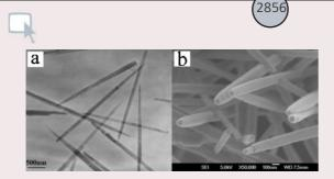
A simple low-temperature growth of ZnO nanowhiskers directly from aqueous solution containing  $Zn(OH)_4^{2-}$  ions
